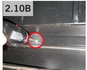
**NOTE:** Check that wiring and harnesses are secured and routed properly in machine cabinet. Inspect wiring and harnesses for any potential pinch points along door and inner door frame.
