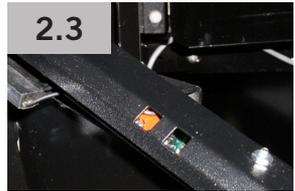
**NOTE:** Ensure sensor bracket assembly is not tilted or twisted after mounting.
