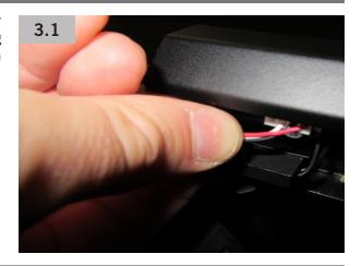
**NOTE:** Ensure drop sensor assembly is not tilted or twisted after mounting.
