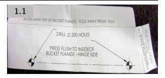
**NOTE:** It is highly recommended to use tape when mounting the template to the drop sensor mounting bracket. If tape is unavailable, hold template firmly in place and have another person mark the template and bracket.
