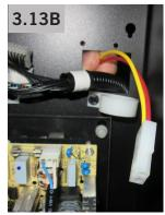
3.14 Connect female end of power adapter harness from rectangular cutout to power supply board connector as shown in **FIG. 3.14**.
