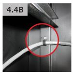
4.5 Pull power supply cable through cutout. Then, connect 24V power supply to power supply board as shown in **FIG. 4.5**.
