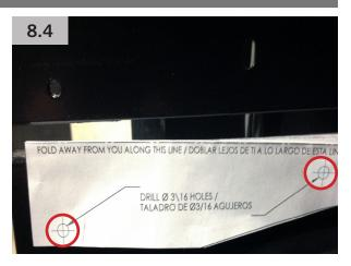
8.5 Using 3/16" drill bit, drill two holes on drop sensor mounting bracket in two locations from marks in Step 8.4 (**FIG. 8.5**).
