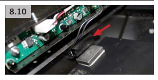
8.11 Move delivery bucket up and down. Green light (LED) on sensor board should illuminate when door is open and turn off when door is closing. Adjust magnet to achieve desired result. When proper placement is identified, remove backing on two-sided tape and apply firmly to delivery bucket door. Refer to **FIG. 8.10**.
