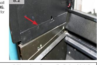
**NOTE:** It is highly recommended to use tape when mounting the template to the drop sensor mounting bracket. If tape is unavailable, hold template firmly in place and have another person mark the template and bracket.
