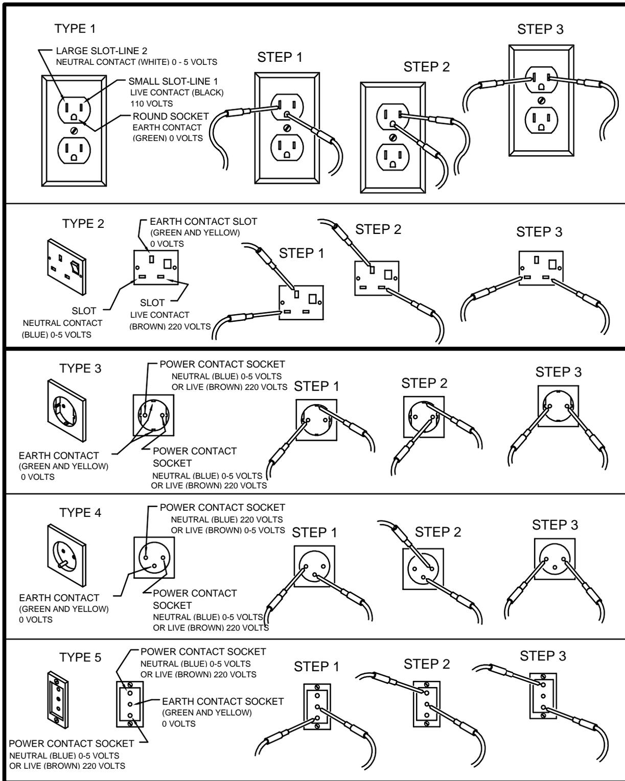
FIGURE 1 CHECKING FOR PROPER GROUNDING AND POLARIZATION
