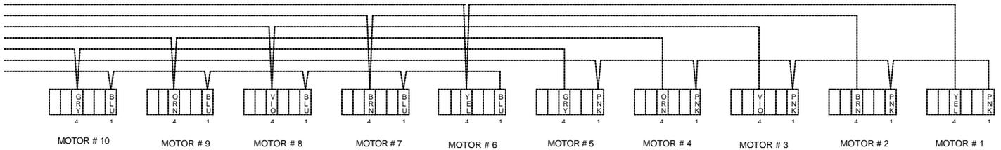
**PINS 1&4: 12VDC MOTOR ACTIVATE / SWITCH MONITOR CIRCUIT (2X5 MATRIX)**
