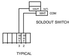
**PINS 2&3: 0 VDC SOLDOUT SWITCH TO MOTOR BOARD (EXTENSION OF 2X5 MATRIX)**
