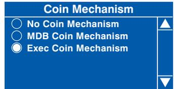
2. Press the ↵ (Edit) key to save the selection and return to the Monetary menu. Verify that the chosen coin mechanism option is displayed in the status line at the bottom of the display.
