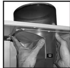
Fill the container with fresh coffee beans. The container has a capacity of approximately 4.0 lbs (1.8 kgs). Refit the cover ensuring that the clips are located correctly.
