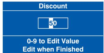
**Note:** When machine is fitted with a coin mechanism, please ensure that discount value entered can be supported by the coin tubes.
