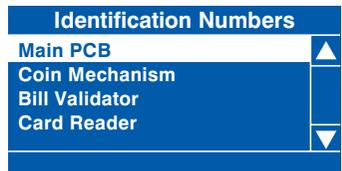
**Note:** Coin Mechanism, Bill Validator and Card Reader will only be displayed if an MDB device is fitted to the machine.
