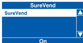
2. To disable SureVend™, press the ↵ (Edit) key to enter the SureVend On/Off screen. Use the ▲ (up) key to select Off (indicated by the filled radio button).
