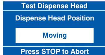
2. When the head reaches its first dispense position, it will stop and the LCD screen will show the message **Dispense Head Position - Extended**. Press the START key a second time to move the head to its second dispense position. Press the START key again to move the head to its fully extended dispense position.
