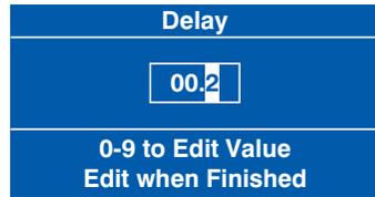
Press the ↵ (Edit) key and verify that the status line confirms that Delay (when highlighted) is set to 0.2hrs.
