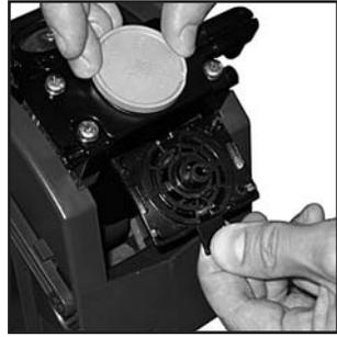
4. Using a 3mm allen key, remove the bolt securing the brewer drive coupling to the input shaft. Pull the coupling off of the shaft and place to one side.
