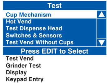
**1. Cup Mechanism:** This sub menu allows the engineer to test the operation of the cup drop unit and replicates the function assigned to switch 7 on the service keypad (see page 56).
