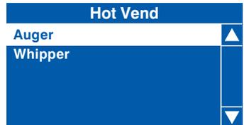
**1. Auger:** This sub menu allows the engineer to test for correct operation of each individual ingredient motor fitted to the machine. Press the ↵ (Edit) key to display the test screen which indicates the number of motors fitted to the machine.
