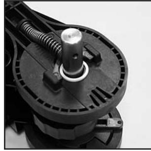
12. Re-fit the brewer drive coupling to the input shaft ensuring that the raised 'pip' (b) lines up with its locating dimple (c) on the input shaft.
