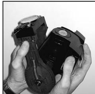
7. Take the new lower piston and cylinder assembly from the service kit.
