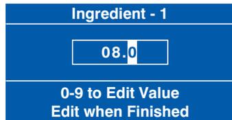
6. Press the ↵ (Edit) key to access the screen as shown. Enter a value for a stronger normal selection, e.g. 8.0 g. Press the sequence 0-8-0 using the drink selection keypad.
