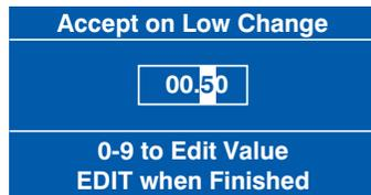
2. Press the ↵ (Edit) key to save the new value and return to the Monetary menu. Verify that the entered value is displayed in the status line at the bottom of the display when Accept on Low Change is highlighted.
