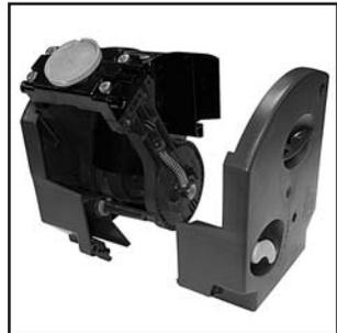
6. Holding the unit as shown in the photograph, rotate the lower piston and cylinder assembly clockwise and then remove it up and out of the swing arms/filter holder assembly.
