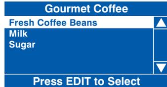
4. With **Fresh Coffee Beans** highlighted press the ↵ (Edit) key to access the menu. The status line at the bottom of the screen shows the current value of the highlighted timer. In the example shown, the Hot Water value is configured to deliver 120ml of water during the vend.
