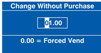
2. Press the ↵ (Edit) key to save the new value and return to the Monetary menu. Verify that the entered value is displayed in the status line at the bottom of the display when Change Without Purchase is highlighted.
