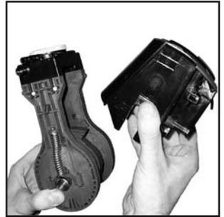
10. Check and ensure that the lower piston guide block (c) locates with the piston drive cam (d) as shown in the photograph.
