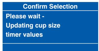
5. Once the software has completed updating the timer values the screen will change and display the message **Update Complete**. Press the ✕ (Exit) key twice to return to the Product Configuration screen.
