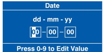
Pressing the **↵** (Edit) key will move back to the Clock menu screen and save the date to the machines memory. Confirm that the status line at the bottom of the screen displays the correct date when Date is highlighted.
