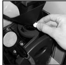
Take one cleaning tablet (supplied in packs of 30 - CMS part no. ZC10598000) and place it into the brewer piston chamber as shown.
