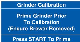
3. The LCD will now display the menu screen as shown opposite. Place the calibrated cup under the grinder outlet and press the START key. The grinder will run and dispense dry ground coffee into the cup.
