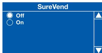
3. Press the ↵ (Edit) key to confirm the selection and return to the SureVend screen. Verify that the status line at the bottom of the screen displays Off when SureVend is highlighted.
