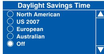
By default daylight savings time is set to Off. To choose one of the available options, press the ▲ (up) or ▼ (down) key until selected (indicated by the filled radio button) followed by the ↵ (Edit) key. Ensure that the required setting is displayed in the status line at the bottom of the screen. Press the X (Exit) key to return to the main menu.
