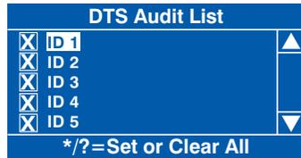
All data and events fields within a vending machine are assigned a unique code determined by the Standard. From this sub-menu the engineer can choose to allow all fields to be available for download by pressing the START/? key or scrolling through the list and adding an X to the required fields.
