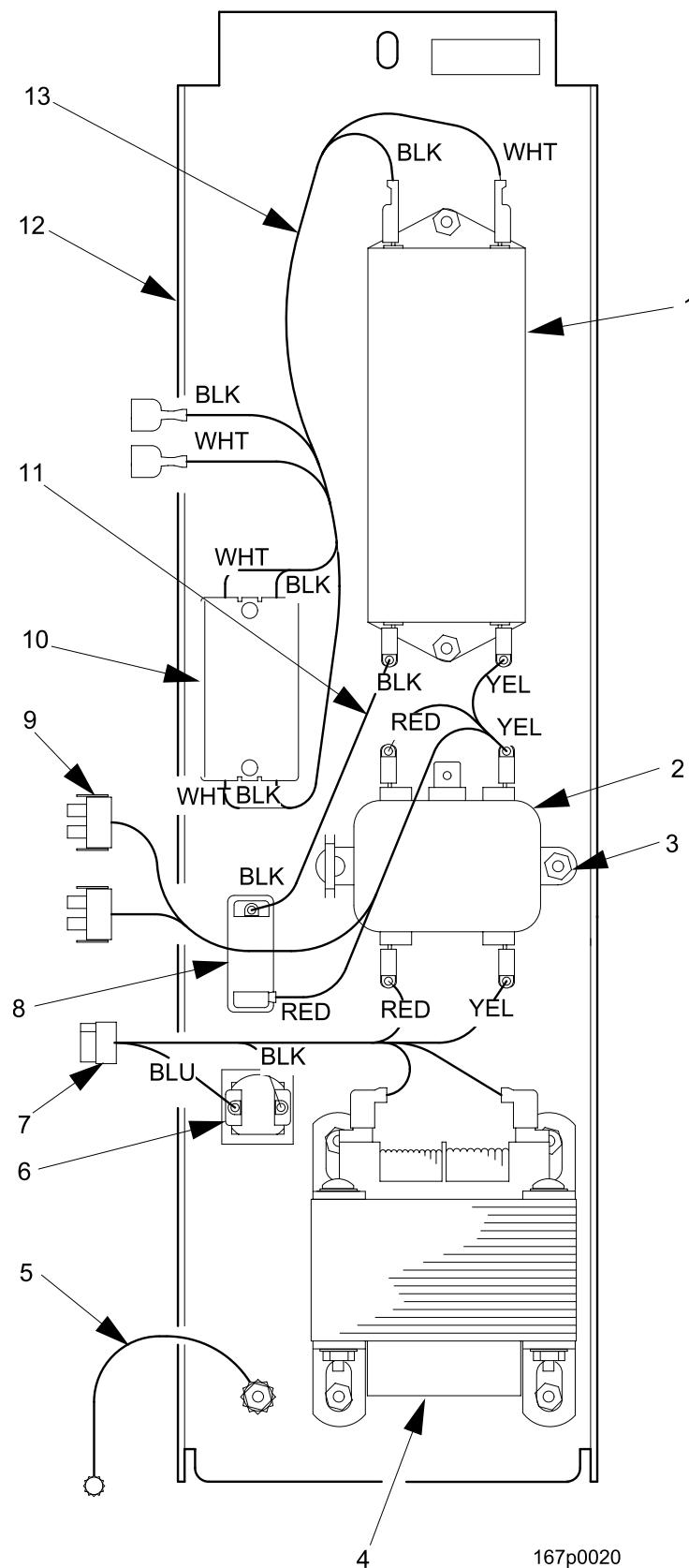
FIGURE 30: POWER PANEL ASSEMBLY - 100V-50/60HZ (JAPAN)
