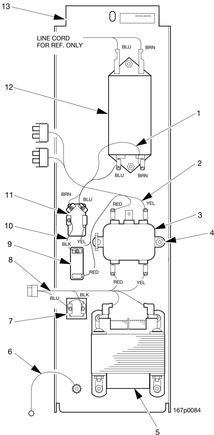
**FIGURE 28: POWER PANEL ASSEMBLY - MODELS 167 168 457 458 - U.K. - 230 V**
