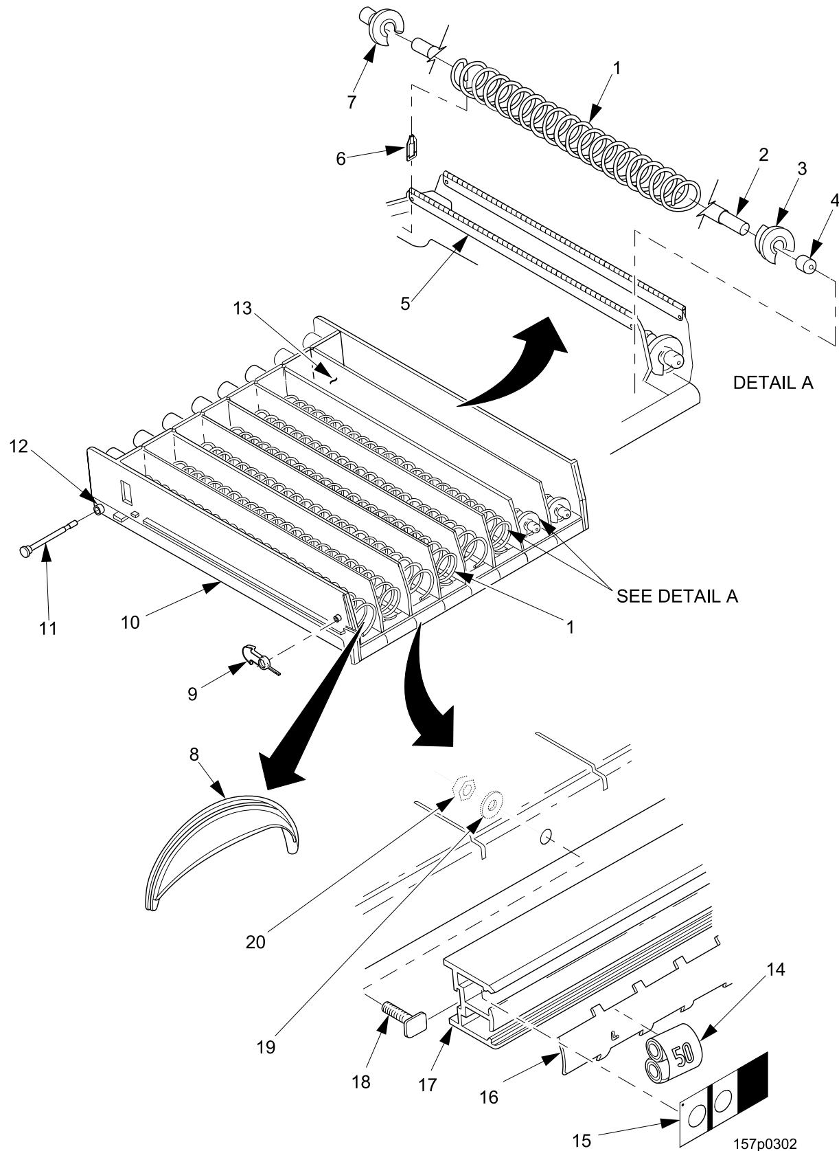
FIGURE 37: GUM AND MINT TRAY ASSEMBLY - 4 MOTOR
