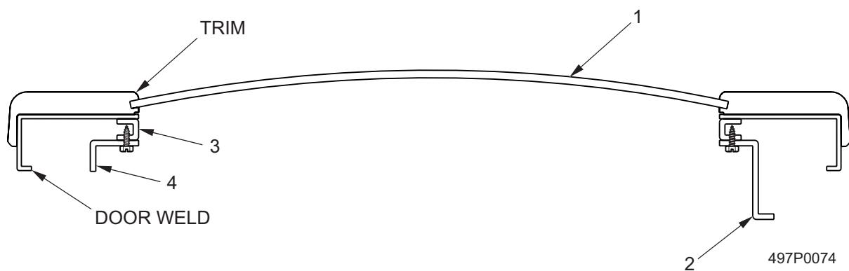
**FIGURE 7: DOOR GLASS AND GLASS RETAINING COMPONENTS (MILLENNIA STYLING)**
