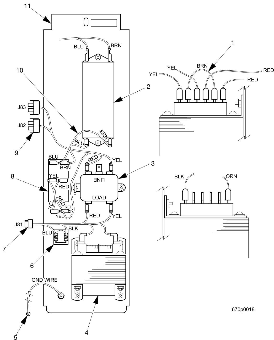
**FIGURE 29: POWER PANEL ASSEMBLY - 230 V - FRANCE / GERMANY**
