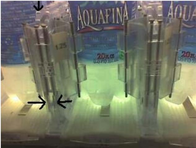
Wiggle the top of the gate and look for cracks.
