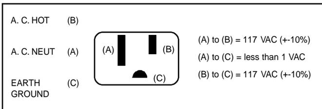
**NOTE: Should the readings be different from above, have a certified electrician correct the problem.**
