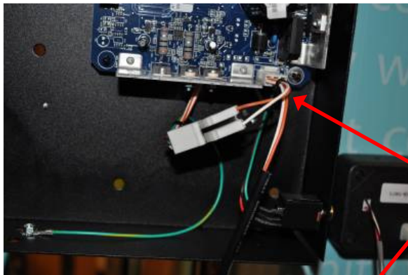
11) Remove factory LED wiring harness from main control board
