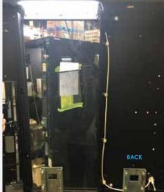
Step 17: Re-install lighted display back on to the door, and re-install machine's cup turrets.
