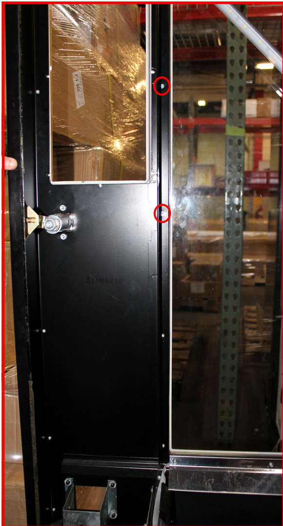
Figure 1 Red circles mark which screws you will be replacing.
