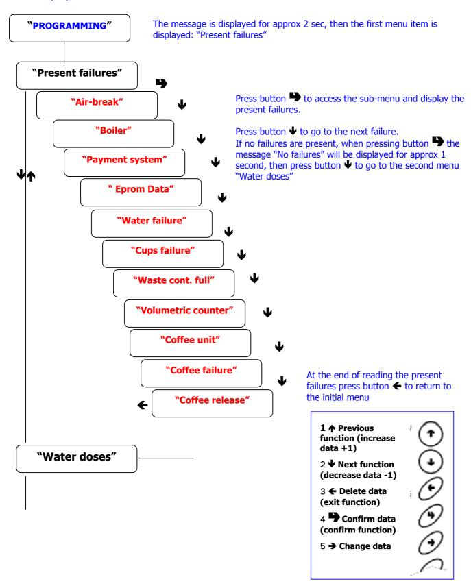
With the display showing the message "Water doses" or "Powder doses" press button → to display the sub-menu "DC xxxx", then press button → to access the relevant sub-menu and the values start blinking, press button → or → to increase or decrease the value by one unit; after reaching the desired value, press button → to confirm the choice, press the button again to return to the initial menu. Press button ← to go back to the previous menu.
