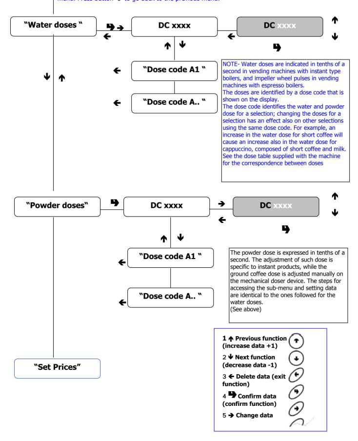
With the display showing the message "Set Prices" press button → to display the sub-menu "Price N. 1", then press button → to access the relevant sub-menu and the values start blinking, press button → or → to increase or decrease the value by one unit; after reaching the desired value, press button → to confirm the choice, press the button again to return to the initial menu. Press button ← to go back to the previous menu.
