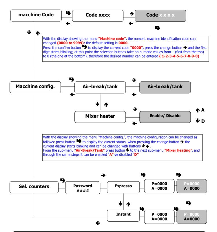
With the display showing the menu **"Selection counter"**, a machine lock can be set, to be triggered after a desired number of espresso coffee or instant product selections.
