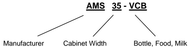
**Example: AMS35 VCB** means it is an Automated Merchandising Systems merchandiser, **35"** wide, with the cabinet trays and columns configured for food, bottles and/or milk –VCB or VCF.
